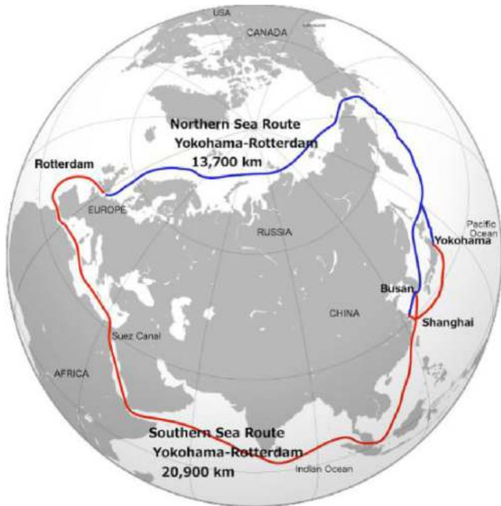
Fig 3: Distance advantage of the NSR (NEP) over the Suez route. Source: Bekkers et al., 2015.
